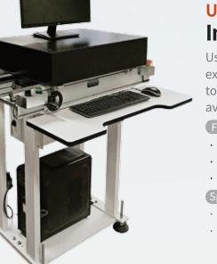
Users can set up a barcode inspection station based on sizes of the existing production lines. Using the image scanning technology together with the analyzation technique, users are able to inspect availability of products fast and thus enhance the quality control.
